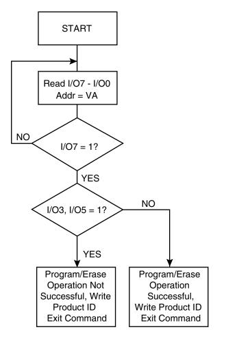
Note: 1. VA = Valid address for programming. During a sector erase operation, a valid address is any sector address within the sector being erased. During chip erase, a valid address is any non-protected sector address.
