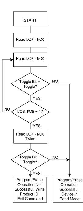
Note: 1. The system should recheck the toggle bit even if I/O5 = "1" because the toggle bit may stop toggling as I/O5 changes to "1".
