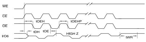
Notes: 1. Toggling either  $\overline{OE}$  or  $\overline{CE}$  or both  $\overline{OE}$  and  $\overline{CE}$  will operate toggle bit.
