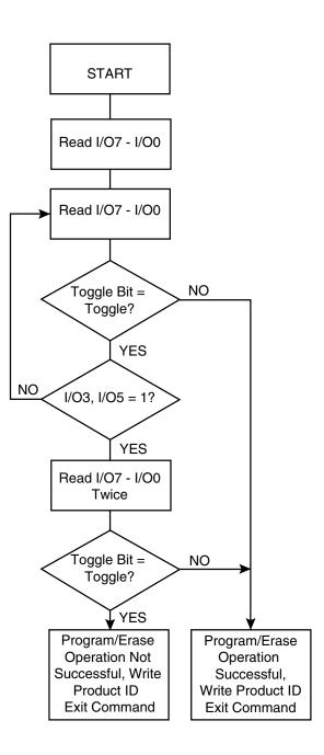
Note: 1. The system should recheck the toggle bit even if I/O5 = "1" because the toggle bit may stop toggling as I/O5 changes to "1".
